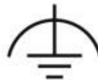
Connection of the protective equipotential bonding conductor
