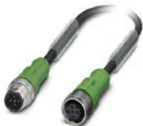
Sensor/actuator cable, 5-position, PUR halogen-free, black-gray RAL 7021, Plug straight M12, coding: A, on Socket straight M12, coding: A, cable length: 3 m
