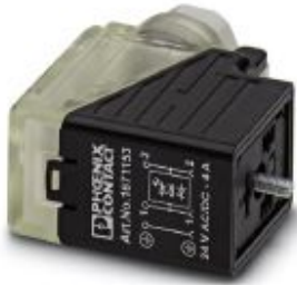
Valve connectors, Universal, 3-position, Valve connector B (10 mm), with 1 LED, connected with Zener diode, Screw connection, cable gland Pg9, external cable diameter 6 mm ... 8 mm
