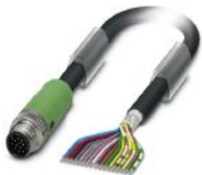
Sensor/actuator cable, 17-position, PUR/PVC, black RAL 9005, shielded, Plug straight M12 SPEEDCON, coding: A, on free cable end, cable length: 10 m
