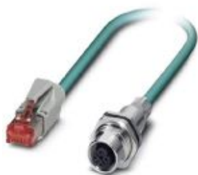
Assembled Ethernet cable, CAT5e, shielded, 2-pair, 26 AWG stranded (7-wire), RAL 5021 (water blue), M12 flush-type socket, rear/screw mounting with SPEEDCON to RJ45 plug/IP20, line, length 0.5 m
