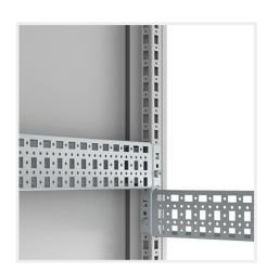
**Opis:** Universal profile for both depth and width fitting on the 25 mm DIN hole pattern of the enclosure's frame or in combination with the CLPF and VB profiles. The 75 mm wide profile is equipped with three rows of holes of which one is turned 90°. This makes it possible to mount the CLPF profiles in both directions. The CLPK can be secured by the use of self tapping screws.
