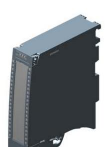
SIMATIC S7-1500, digital output module DQ 32x24 V DC/0.5 A HF; 32 channels in groups of 8; 4 A per group; Single-channel diagnostics; Substitute value: Front connector (screw terminals or push-in) to be ordered separately
