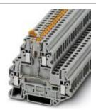
Knife disconnect terminal block, With test socket screws for insertion of test plugs, nom. voltage: 24 V, nominal current: 30 A, connection method: Screw connection, cross section: 0.14 mm² - 6 mm², AWG: 26 - 10, length: 69.9 mm, width: 6.2 mm, color: gray, mounting: NS 35/7,5, NS 35/15
