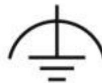
Connection of the protective equipotential bonding conductor
