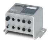
PoE+ Ethernet switch, 8 Ethernet ports in M12 format, automatic detection of the data transmission speed of 10/100/1000 Mbps, jumbo frames up to 9600 bytes, coupling of network segments with different transmission speeds, autocrossing function, degree of protection IP67
