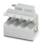
PCB headers, nominal cross section: 2.5 mm², color: light gray, nominal current: 12 A, rated voltage (III/2): 320 V, contact surface: Tin, type of contact: Male connector, Number of potentials: 4, Number of rows: 1, Number of positions per row: 4, number of connections: 4, product range: MSTBO 2,5/..-G1L, pitch: 5 mm, mounting: Wave soldering, pin layout: Linear pinning, solder pin [P]: 3.5 mm, Locking: without, type of packaging: packed in cardboard, Product with pin output on left side
