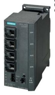
SCALANCE X204IRT, managed IE IRT switch, 4x 10/100 Mbit/s RJ45 ports, Error signaling contact with set pushbutton, redundant power supply, PROFINET IO device, network management, Redundancy Manager integrated, incl. electron. manual on CD-ROM, C-plug optional
